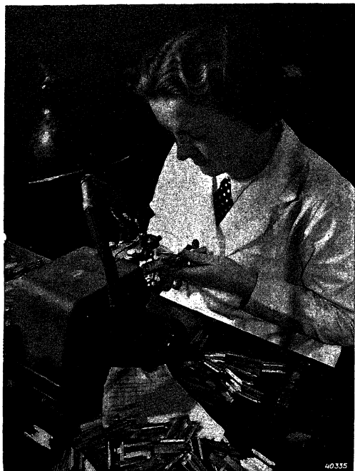
Fig. 69 Spot-welding the supports to anodes and screen plates.
